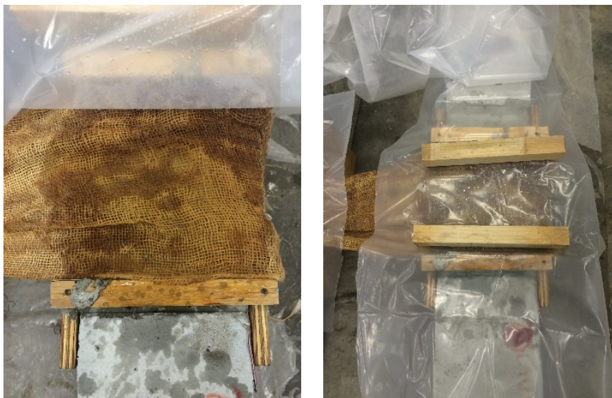
Figure 5.20 Curing using burlap
