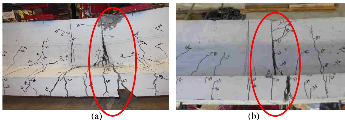
Figure 6.24 Failure mode (a) B-4-U-MB-M (b) B-5-U-U-M
