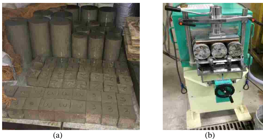
Figure 5.16 (a) Cube and cylinder specimens (b) end grinder
