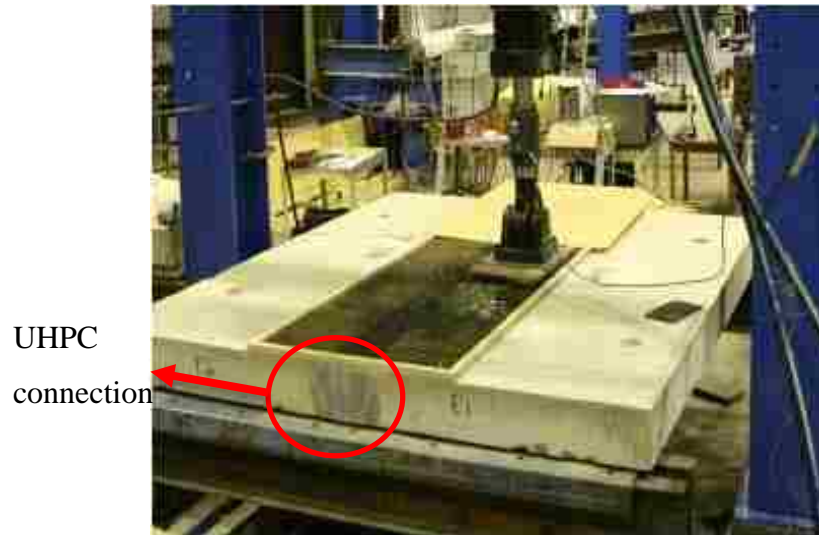
Figure 2.5 Test setup used in FHWA study HRT-11-023
