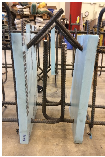
Figure 3.12 (a) MoDOT end girder detail in Highway-50, (b) non-prestressed Joint detail
